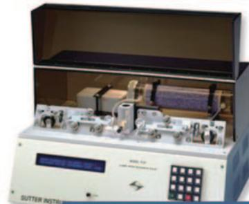
P-97 Micropipette Puller
