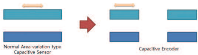
Figure 3 Capacitive encoder
